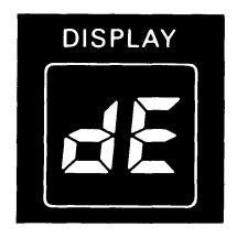
This flashing code tells you something's wrong with the defrost system—keep doors closed to retain cold and call for service. Code flashes until problem is corrected.
